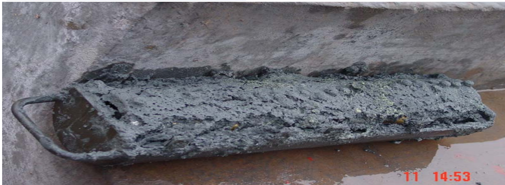
Sulfur plugging of some wells in Sichuan basin ( H_2S 6.87%, CO_2 2.76%)
